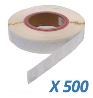
This NFC sticker is a 25mm diameter white sticky label that operates at 13.56 MHz wireless frequency and contains 137 bytes of usable read/write space for NDEF data. Based on the NTAG213 chip from NXP, this sticker offers advanced security, anticloning features as well as a permanent lock feature, therefore user data can be permanently configured read-only. The NTAG213 NFC chip features improved performance and is fully backwards compatible with NTAG203 and MIFARE Ultralight C.
